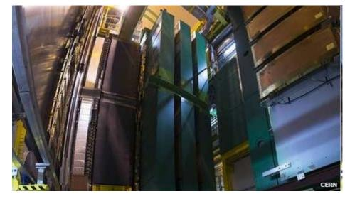
Detectors positioned at key points around the underground "ring" are then used to scour the wreckage of these collisions for signs of new particles and physical phenomena.
